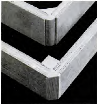
SOLID-WOOD INSETS , used with glue-block backing, produce corners that are both distinctive and strong. The insets may be square or triangular, round or cove. Recessed or raised insets will heighten the decorative effect.
